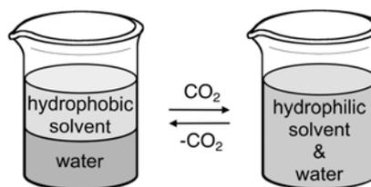
Fig. 2 – Switchable-hydrophilicity solvents, such as CyNMe<sub>2</sub>, normally form a biphasic mixture when mixed with water, but will react with CO<sub>2</sub> to make a bicarbonate salt that is soluble in water, thus causing the two liquid phases to merge into one. Removal of the CO<sub>2</sub> reverses the process.
