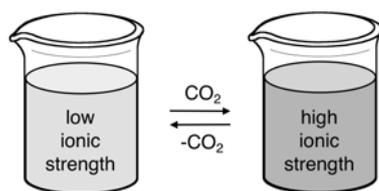
Fig. 3 – Switchable water is an aqueous solution of switchable ionic strength. The solution of an amine or polyamine in water has very low ionic strength, but if CO<sub>2</sub> is introduced the polyamine is converted into a bicarbonate salt (polyelectrolyte), causing the ionic strength of the solution to jump dramatically. Removal of the CO<sub>2</sub> reverses the process.
