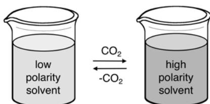
Fig. 1 – Switchable-polarity solvents, such as secondary amines or amidine/alcohol mixes, react with CO<sub>2</sub> to make a solvent of higher polarity than the original. Removal of the CO<sub>2</sub> reverses the process.
