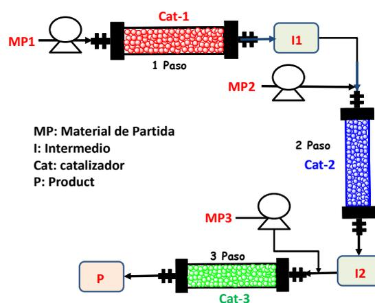
Fig.2 Multireactor network for the synthesis of a product through the integration of three catalytic steps.
