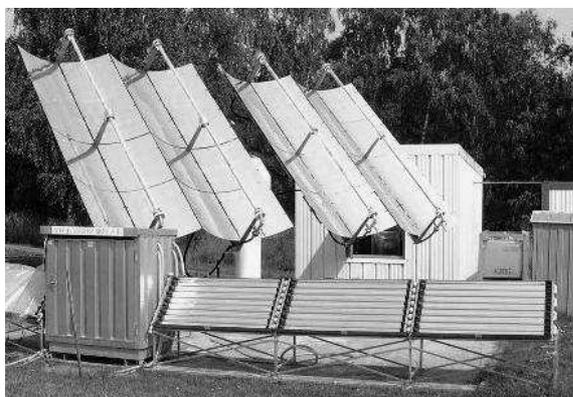
Fig. 1 – PROPHIS (back) and CPC (front) reactors at the German Aerospace Centre (DLR) in Cologne, Germany.
